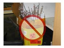
Pipettes and tips that <u>are not contaminated</u> with biological or chemical materials should be placed into a box or other sturdy container lined with a clear plastic bag and disposed of through the normal solid waste.
